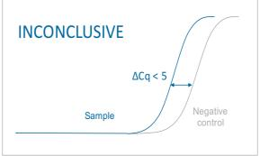
If the sample amplifies > 5 Cq earlier than the negative control then the sample should be reinterpreted (via the table above) with the negative control verified as negative. If the sample amplifies < 5 Cq earlier than the negative control then the positive sample result is invalidated and the result should be determined inconclusive due to test contamination. The test for this sample should be repeated.
